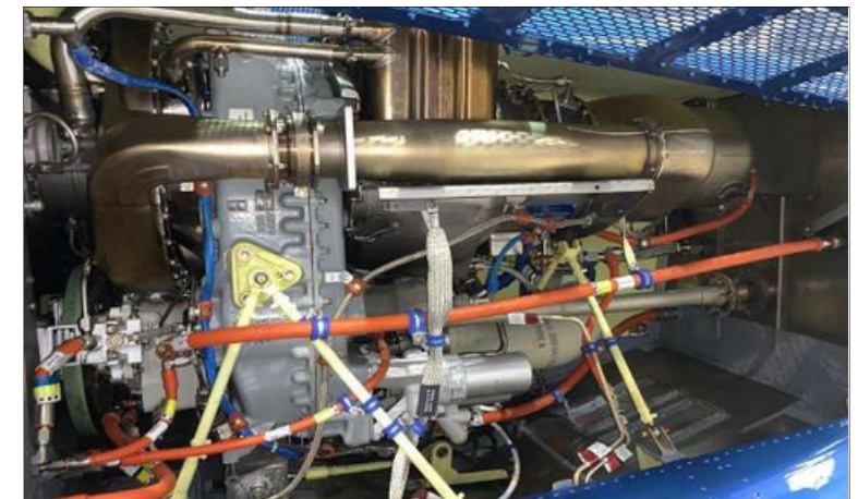
Rolls-Royce 250-C47B/8 Engine with Full Authority Digital Electronic Control
